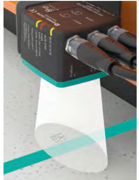
The unique positioning system Position Guided Vision is the first in the world to combine two technologies in one device: optical colored tape/paint tracking for driving and Data Matrix codes for precise position detection of automated guided vehicles.
