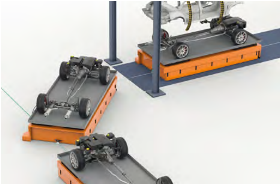
The unique positioning system Position Guided Vision is the first in the world to combine two technologies in one device: optical colored tape/paint tracking for driving and Data Matrix codes for precise position detection of automated guided vehicles.
